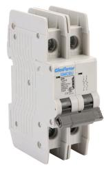
Gladiator miniature circuit breaker, 20A, 480Y / 277 VAC / 125 VDC, 2-pole, B curve, thermal magnetic, 10kA @ 480Y/277 VAC interrupting rating, 35mm DIN rail mount.
