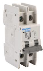
Gladiator miniature circuit breaker, 1A, 480Y / 277 VAC / 125 VDC, 2-pole, B curve, thermal magnetic, 10kA @ 480Y/277 VAC interrupting rating, 35mm DIN rail mount.
