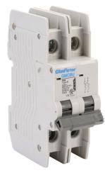
Gladiator miniature circuit breaker, 16A, 480Y / 277 VAC / 125 VDC, 2-pole, B curve, thermal magnetic, 10kA @ 480Y/277 VAC interrupting rating, 35mm DIN rail mount.
