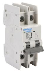
Gladiator miniature circuit breaker, 15A, 480Y / 277 VAC / 125 VDC, 2-pole, B curve, thermal magnetic, 10kA @ 480Y/277 VAC interrupting rating, 35mm DIN rail mount.
