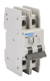
Gladiator miniature circuit breaker, 10A, 480Y / 277 VAC / 125 VDC, 2-pole, B curve, thermal magnetic, 10kA @ 480Y/277 VAC interrupting rating, 35mm DIN rail mount.
