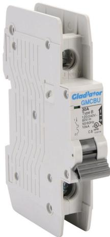
Gladiator miniature circuit breaker, 30A, 240 VAC / 60 VDC, 1-pole, B curve, thermal magnetic, 10kA @ 120/240 VAC interrupting rating, 35mm DIN rail mount.
