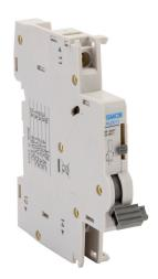
Gladiator auxiliary contact, left side mount, SPDT contact(s), 6A @ 240 VAC/1A @ 110 VDC. For use with Gladiator GMCB series supplementary protectors.
