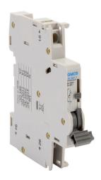
Gladiator alarm contact, left side mount, SPDT contact(s), 6A @ 240 VAC/1A @ 110 VDC. For use with Gladiator GMCB series supplementary protectors.
