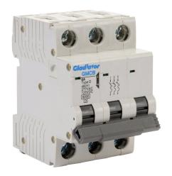
Gladiator miniature supplementary protector, 8A, 480Y / 277 VAC / 125 VDC, 3-pole, D curve, thermal magnetic, 6kA @ 480Y/277 VAC interrupting rating, 35mm DIN rail mount.
