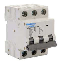
Gladiator miniature supplementary protector, 8A, 480Y / 277 VAC / 125 VDC, 3-pole, D curve, thermal magnetic, 6kA @ 480Y/277 VAC interrupting rating, 35mm DIN rail mount.
