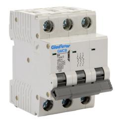
Gladiator miniature supplementary protector, 6A, 480Y / 277 VAC / 125 VDC, 3-pole, D curve, thermal magnetic, 6kA @ 480Y/277 VAC interrupting rating, 35mm DIN rail mount.
