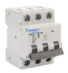
Gladiator miniature supplementary protector, 63A, 480Y / 277 VAC / 125 VDC, 3-pole, D curve, thermal magnetic, 6kA @ 480Y/277 VAC interrupting rating, 35mm DIN rail mount.
