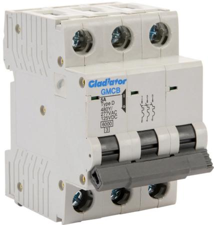
Gladiator miniature supplementary protector, 5A, 480Y / 277 VAC / 125 VDC, 3-pole, D curve, thermal magnetic, 6kA @ 480Y/277 VAC interrupting rating, 35mm DIN rail mount.
