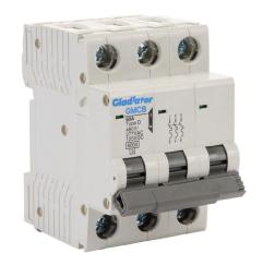
Gladiator miniature supplementary protector, 50A, 480Y / 277 VAC / 125 VDC, 3-pole, D curve, thermal magnetic, 6kA @ 480Y/277 VAC interrupting rating, 35mm DIN rail mount.
