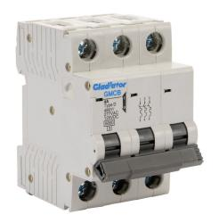
Gladiator miniature supplementary protector, 4A, 480Y / 277 VAC / 125 VDC, 3-pole, D curve, thermal magnetic, 6kA @ 480Y/277 VAC interrupting rating, 35mm DIN rail mount.
