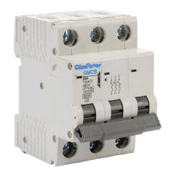
Gladiator miniature supplementary protector, 40A, 480Y / 277 VAC / 125 VDC, 3-pole, D curve, thermal magnetic, 6kA @ 480Y/277 VAC interrupting rating, 35mm DIN rail mount.
