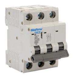
Gladiator miniature supplementary protector, 3A, 480Y / 277 VAC / 125 VDC, 3-pole, D curve, thermal magnetic, 6kA @ 480Y/277 VAC interrupting rating, 35mm DIN rail mount.
