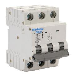
Gladiator miniature supplementary protector, 32A, 480Y / 277 VAC / 125 VDC, 3-pole, D curve, thermal magnetic, 6kA @ 480Y/277 VAC interrupting rating, 35mm DIN rail mount.
