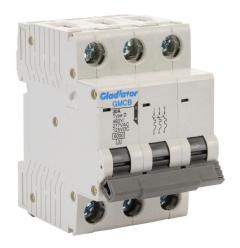
Gladiator miniature supplementary protector, 30A, 480Y / 277 VAC / 125 VDC, 3-pole, D curve, thermal magnetic, 6kA @ 480Y/277 VAC interrupting rating, 35mm DIN rail mount.
