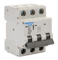
Gladiator miniature supplementary protector, 2A, 480Y / 277 VAC / 125 VDC, 3-pole, D curve, thermal magnetic, 6kA @ 480Y/277 VAC interrupting rating, 35mm DIN rail mount.
