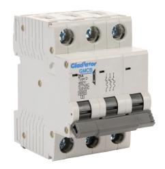
Gladiator miniature supplementary protector, 25A, 480Y / 277 VAC / 125 VDC, 3-pole, D curve, thermal magnetic, 6kA @ 480Y/277 VAC interrupting rating, 35mm DIN rail mount.
