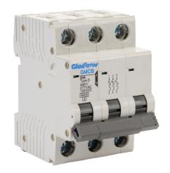
Gladiator miniature supplementary protector, 20A, 480Y / 277 VAC / 125 VDC, 3-pole, D curve, thermal magnetic, 6kA @ 480Y/277 VAC interrupting rating, 35mm DIN rail mount.
