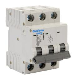
Gladiator miniature supplementary protector, 1A, 480Y / 277 VAC / 125 VDC, 3-pole, D curve, thermal magnetic, 6kA @ 480Y/277 VAC interrupting rating, 35mm DIN rail mount.
