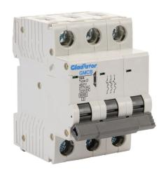
Gladiator miniature supplementary protector, 16A, 480Y / 277 VAC / 125 VDC, 3-pole, D curve, thermal magnetic, 6kA @ 480Y/277 VAC interrupting rating, 35mm DIN rail mount.
