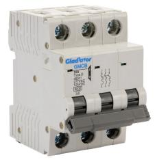
Gladiator miniature supplementary protector, 10A, 480Y / 277 VAC / 125 VDC, 3-pole, D curve, thermal magnetic, 6kA @ 480Y/277 VAC interrupting rating, 35mm DIN rail mount.
