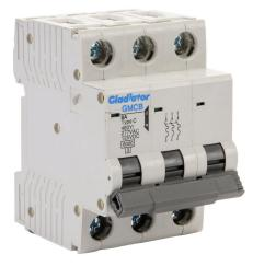
Gladiator miniature supplementary protector, 8A, 480Y / 277 VAC / 125 VDC, 3-pole, C curve, thermal magnetic, 6kA @ 480Y/277 VAC interrupting rating, 35mm DIN rail mount.
