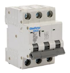
Gladiator miniature supplementary protector, 6A, 480Y / 277 VAC / 125 VDC, 3-pole, C curve, thermal magnetic, 6kA @ 480Y/277 VAC interrupting rating, 35mm DIN rail mount.
