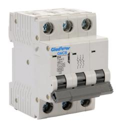
Gladiator miniature supplementary protector, 63A, 480Y / 277 VAC / 125 VDC, 3-pole, C curve, thermal magnetic, 6kA @ 480Y/277 VAC interrupting rating, 35mm DIN rail mount.
