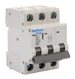
Gladiator miniature supplementary protector, 5A, 480Y / 277 VAC / 125 VDC, 3-pole, C curve, thermal magnetic, 6kA @ 480Y/277 VAC interrupting rating, 35mm DIN rail mount.
