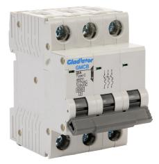
Gladiator miniature supplementary protector, 50A, 480Y / 277 VAC / 125 VDC, 3-pole, C curve, thermal magnetic, 6kA @ 480Y/277 VAC interrupting rating, 35mm DIN rail mount.
