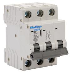
Gladiator miniature supplementary protector, 40A, 480Y / 277 VAC / 125 VDC, 3-pole, C curve, thermal magnetic, 6kA @ 480Y/277 VAC interrupting rating, 35mm DIN rail mount.
