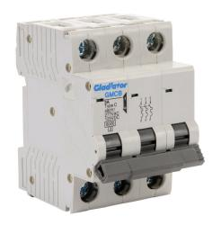
Gladiator miniature supplementary protector, 3A, 480Y / 277 VAC / 125 VDC, 3-pole, C curve, thermal magnetic, 6kA @ 480Y/277 VAC interrupting rating, 35mm DIN rail mount.
