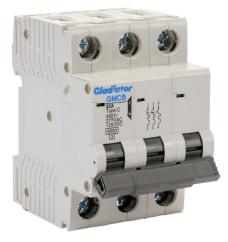
Gladiator miniature supplementary protector, 32A, 480Y / 277 VAC / 125 VDC, 3-pole, C curve, thermal magnetic, 6kA @ 480Y/277 VAC interrupting rating, 35mm DIN rail mount.
