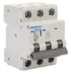
Gladiator miniature supplementary protector, 2A, 480Y / 277 VAC / 125 VDC, 3-pole, C curve, thermal magnetic, 6kA @ 480Y/277 VAC interrupting rating, 35mm DIN rail mount.
