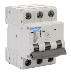
Gladiator miniature supplementary protector, 25A, 480Y / 277 VAC / 125 VDC, 3-pole, C curve, thermal magnetic, 6kA @ 480Y/277 VAC interrupting rating, 35mm DIN rail mount.
