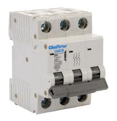
Gladiator miniature supplementary protector, 20A, 480Y / 277 VAC / 125 VDC, 3-pole, C curve, thermal magnetic, 6kA @ 480Y/277 VAC interrupting rating, 35mm DIN rail mount.
