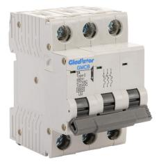
Gladiator miniature supplementary protector, 1A, 480Y / 277 VAC / 125 VDC, 3-pole, C curve, thermal magnetic, 6kA @ 480Y/277 VAC interrupting rating, 35mm DIN rail mount.
