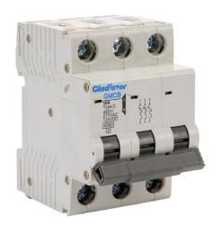
Gladiator miniature supplementary protector, 16A, 480Y / 277 VAC / 125 VDC, 3-pole, C curve, thermal magnetic, 6kA @ 480Y/277 VAC interrupting rating, 35mm DIN rail mount.
