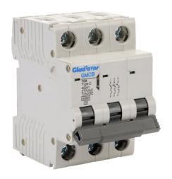
Gladiator miniature supplementary protector, 15A, 480Y / 277 VAC / 125 VDC, 3-pole, C curve, thermal magnetic, 6kA @ 480Y/277 VAC interrupting rating, 35mm DIN rail mount.
