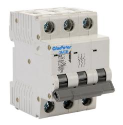
Gladiator miniature supplementary protector, 10A, 480Y / 277 VAC / 125 VDC, 3-pole, C curve, thermal magnetic, 6kA @ 480Y/277 VAC interrupting rating, 35mm DIN rail mount.
