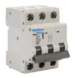
Gladiator miniature supplementary protector, 8A, 480Y / 277 VAC / 125 VDC, 3-pole, B curve, thermal magnetic, 6kA @ 480Y/277 VAC interrupting rating, 35mm DIN rail mount.
