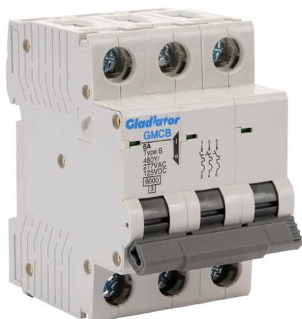
Gladiator miniature supplementary protector, 6A, 480Y / 277 VAC / 125 VDC, 3-pole, B curve, thermal magnetic, 6kA @ 480Y/277 VAC interrupting rating, 35mm DIN rail mount.
