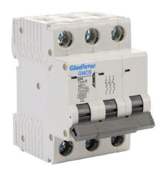
Gladiator miniature supplementary protector, 63A, 480Y / 277 VAC / 125 VDC, 3-pole, B curve, thermal magnetic, 6kA @ 480Y/277 VAC interrupting rating, 35mm DIN rail mount.
