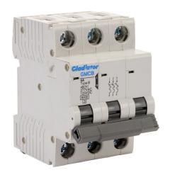
Gladiator miniature supplementary protector, 5A, 480Y / 277 VAC / 125 VDC, 3-pole, B curve, thermal magnetic, 6kA @ 480Y/277 VAC interrupting rating, 35mm DIN rail mount.
