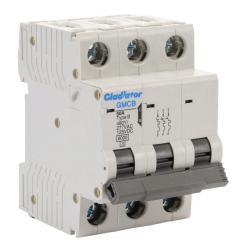
Gladiator miniature supplementary protector, 50A, 480Y / 277 VAC / 125 VDC, 3-pole, B curve, thermal magnetic, 6kA @ 480Y/277 VAC interrupting rating, 35mm DIN rail mount.
