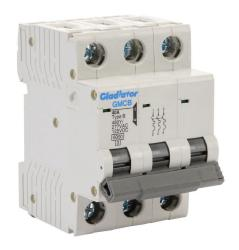
Gladiator miniature supplementary protector, 40A, 480Y / 277 VAC / 125 VDC, 3-pole, B curve, thermal magnetic, 6kA @ 480Y/277 VAC interrupting rating, 35mm DIN rail mount.
