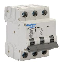
Gladiator miniature supplementary protector, 3A, 480Y / 277 VAC / 125 VDC, 3-pole, B curve, thermal magnetic, 6kA @ 480Y/277 VAC interrupting rating, 35mm DIN rail mount.
