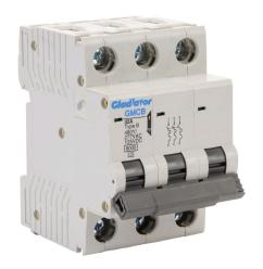
Gladiator miniature supplementary protector, 32A, 480Y / 277 VAC / 125 VDC, 3-pole, B curve, thermal magnetic, 6kA @ 480Y/277 VAC interrupting rating, 35mm DIN rail mount.
