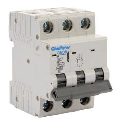
Gladiator miniature supplementary protector, 2A, 480Y / 277 VAC / 125 VDC, 3-pole, B curve, thermal magnetic, 6kA @ 480Y/277 VAC interrupting rating, 35mm DIN rail mount.
