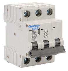
Gladiator miniature supplementary protector, 25A, 480Y / 277 VAC / 125 VDC, 3-pole, B curve, thermal magnetic, 6kA @ 480Y/277 VAC interrupting rating, 35mm DIN rail mount.
