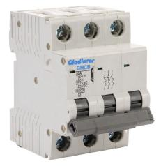
Gladiator miniature supplementary protector, 20A, 480Y / 277 VAC / 125 VDC, 3-pole, B curve, thermal magnetic, 6kA @ 480Y/277 VAC interrupting rating, 35mm DIN rail mount.
